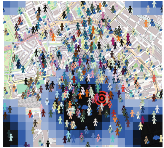
Figure 2: Visualisation of data aggregation. Lines between users (not to scale) indicate data aggregation, adjacent users with the same colour indicate a cluster where only one in that cluster is providing data. Rainclouds are indicated with blue and black squares. Map taken from ©OpenStreetMap.
